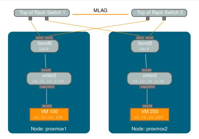
Another possibility it to use the bond directly as bridge port. This can be used to make the guest network fault-tolerant.
