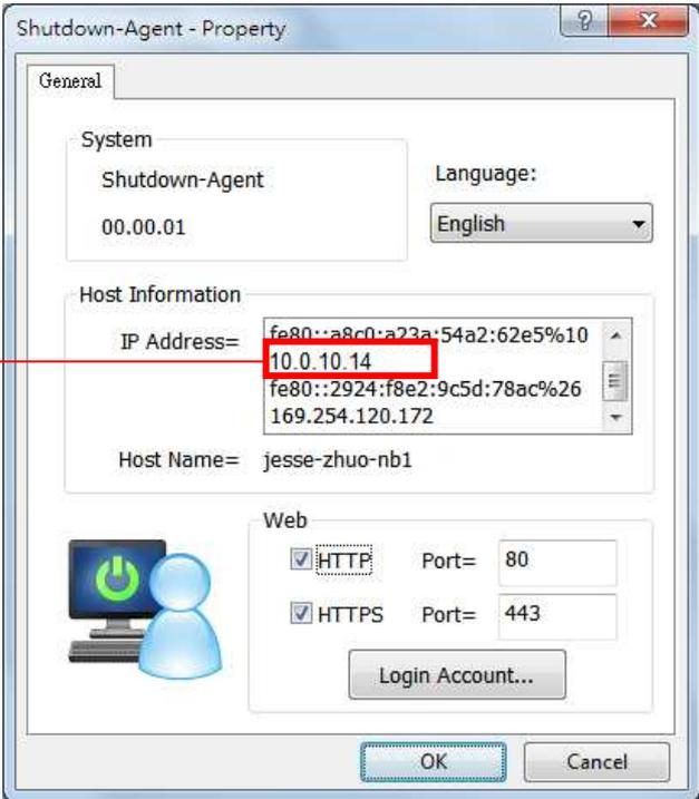
5. Back to the InsightPower SNMP IPv6 card web page, add the IP address of ShutdownAgent to the SNMP Trap table. Please select the "ShutdownAgent 2012" for the Event Level and UPSV4 or UPSv5 as the Trap MIB.
