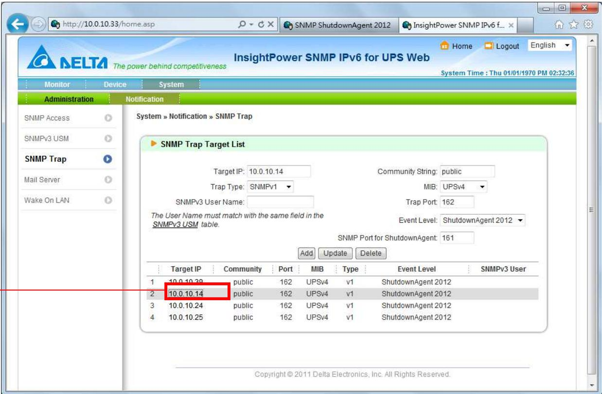
6. If you enable the manageable option in the ShutdownAgent then you can observe all of the shutdown status, countdown timer and shutdown reason from the InsightPower SNMP IPv6 card. The web page is on the Monitor >> Information >> ShutdownAgent.
