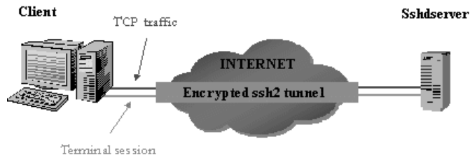
Figure 2.1: Making insecure TCP connections secure using channels inside the encrypted ssh2 tunnel
